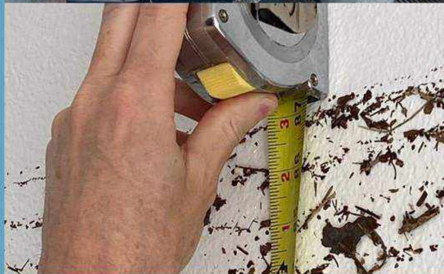
Hurricane Ian (Cat 4) 11.5 ft AGL storm surge in Fort Myers Beach, FL
